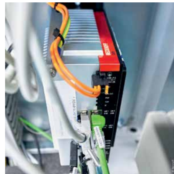
The C6030 ultra-compact Industrial PC serves as the powerful control core of the BLS 500 and requires very little installation space.
