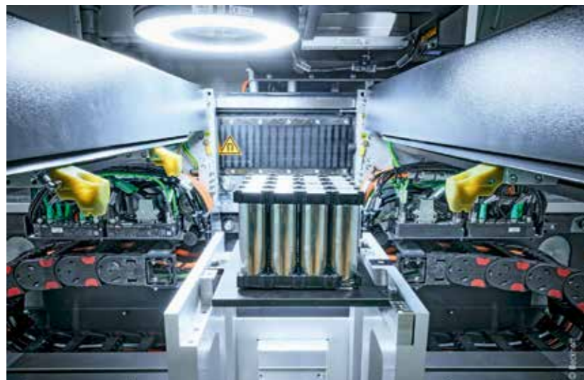
With its modular and flexible design, the BLS 500 laser welding system from Manz can be adapted to a wide variety of applications, such as the manually fed battery module shown here.
