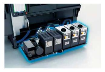
designed machine enclosure ensures best accessibility to all components. To allow best accessibility for maintenance, all temperature control units and the vacuum pump are positioned on a retractable service rack. In addition, the machine enclosure and frame has been configured such that conveyor belts can be installed on any of 3 machine sides for utmost flexibility and use of automation.
